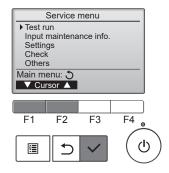
2. Select "Test run" with the F1 or F2 button, and press the [ ✓ ] button.
