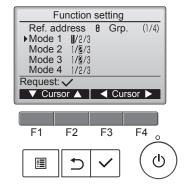
5. When the settings are completed, press the [ ✓ ] button to send the setting data from the remote controller to the indoor units.
