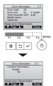
2. Press the  $\boxed{\mathsf{F4}}$  button or the  $\binom{0}{2}$  button to reset the error that is occurring.
