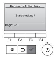
3. OK: No problems are found with the remote controller. Check other parts for problems.
