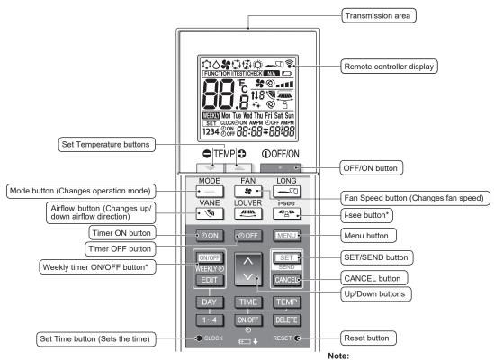
This button is enabled or disabled depending on the model of the indoor unit.
