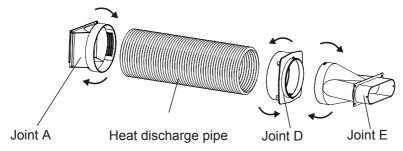
Insert joint A of heat discharge pipe (the side with "TOP" is upwards) into the groove until you hear a sound.
