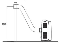
• Wrong installation is shown in following figure (If the pipe is bent too much, it would easily cause malfunction.)
