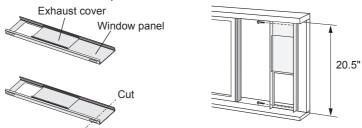
Inner height of the window:20.5" (520mm)- 38.5" (980mm) Use the window panel and the adjustment panel.
