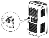
2. Screw the drain connector to(included in the package) the spout by turning clockwise.
