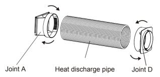
2. Insert joint A of heat discharge pipe (the side with "TOP" is upwards) into the groove until you hear a sound.
