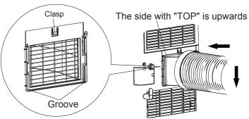
Slide and open the exhaust cover on the window panel, and attach the window adapter.
