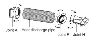
3. Insert joint A of heat discharge pipe (the side with "TOP" is upwards) into the groove until you hear a sound.
