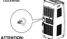
3. Insert the drainage hose into drain connector.
