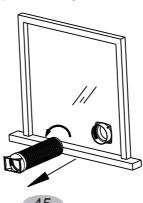
3. When heat discharge pipe is removed, Install the plastic cover into joint F in case of the insect into the house .
