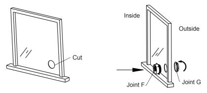
3. Install the other side of heat discharge pipe clockwise into joint F.
