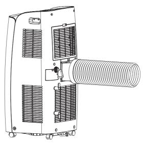
• Correct installation is as shown in figure (When installing it on wall, height of hall should not be over 130cm from floor).
