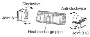
Insert joint A of heat discharge pipe (the side with "TOP" is upwards) into the groove until you hear a sound.
