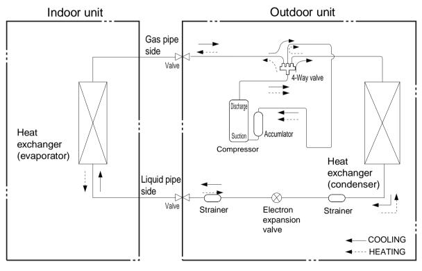
Connection pipe specification: Liquid pipe: 1/4" Gas pipe: 3/8" for 07K / 09K / 12K / 18K(XB) 1/2" for 18K(XD) / 24K(XE) 5/8" for 24K(XF)
