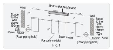
(2) When installation is finished, pull the mounting plate with hand to confirm whether it is fixed tightly. The force distribution for all screws should be uniform.
