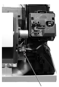
Fixing band of the vane motor wire
