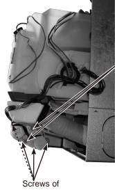
Screws of the vane motor unit cover
