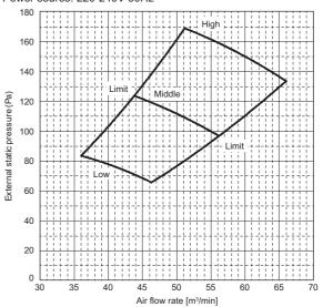
**PEA-M200LA** External static pressure: 200Pa Power source: 220-240V 50Hz
