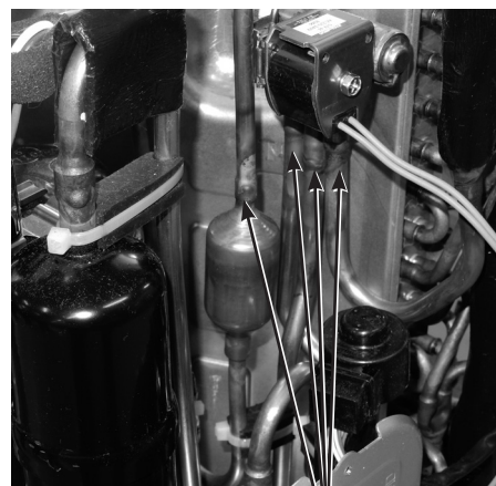
Brazed parts of 4-way valve
