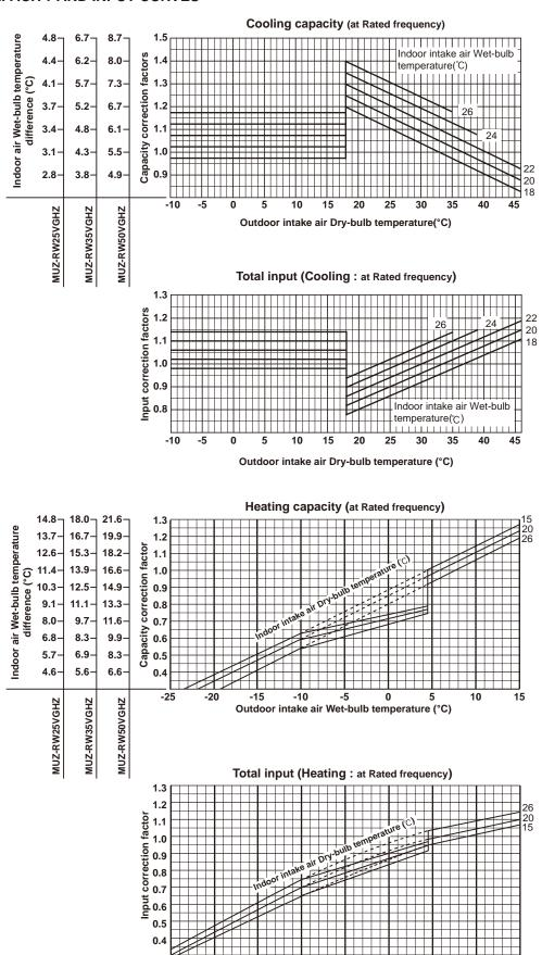
NOTE: The above broken lines are for the heating operation without any frost and defrost operation.
