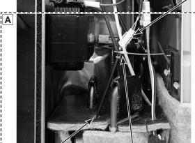
Pass the lead wire of compressor protector through the top felt hole.
