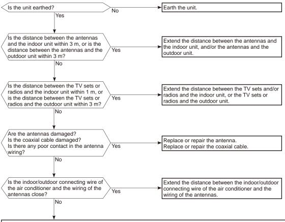
Even if all of the above conditions are fulfilled, the electromagnetic noise may enter, depending on the electric field strength or the installation condition (combination of specific conditions such as antennas or wiring). Check the following before asking for service.
