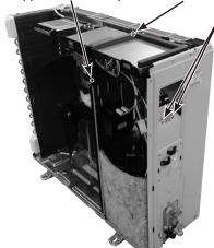
Screws of the terminal block support and the back panel
