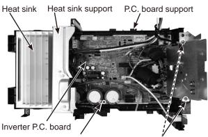
Screw of the inverter P.C. board
