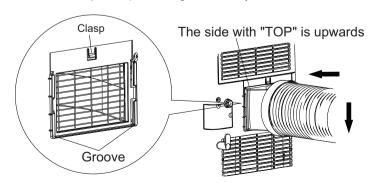
10. Slide and open the exhaust cover on the window panel, and attach the window adapter.
