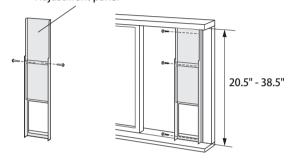
Inner height of the window:38.5" (980mm) - 59" (1500mm) Use the window panel, the adjustment panel and the extension panel.
