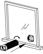
4.Insert joint A of heat discharge pipe (the side with "TOP" is upwards) into the groove until you hear a sound.
