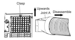
2. Remove the window adapter. Pull out and remove the window adapter by pushing down two "PUSH" markings, and slide and close the exhaust cover in the window panel. (Optional)
