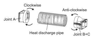
9. Insert joint A of heat discharge pipe (the side with "TOP" is upwards) into the groove until you hear a sound.
