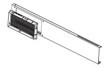
2. Cut the sponge A (adhesive type) to the proper length and attach it to the window stool and to the bottom of sash.
