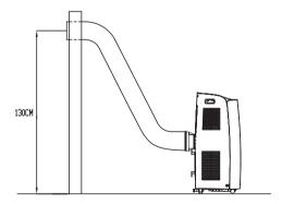
• Wrong installation is shown in following figure (If the pipe is bent too much,it would easily cause malfunction.)
