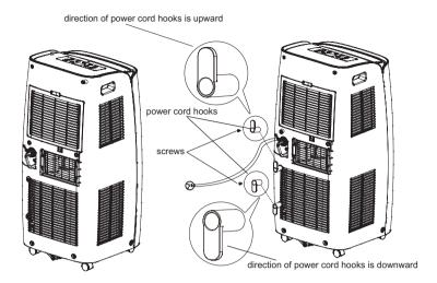
• Wind the power cord around the power cord hooks.
