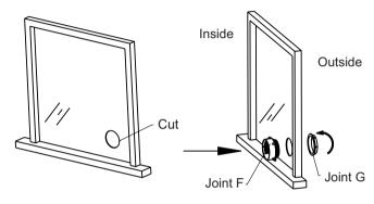
3.Install the other side of heat discharge pipe clockwise into joint F.
