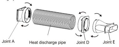
2. Insert joint A of heat discharge pipe (the side with "TOP" is upwards) into the groove until you hear a sound.
