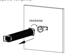
3. When heat discharge pipe is removed, Install the plastic cover into joint D in case of the insect into the house.
