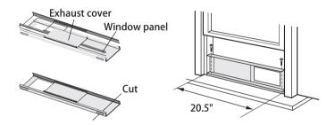
Inner width of the window:20.5" (520mm)- 38.5" (980mm) Use the window panel and the adjustment panel.
