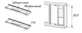
Inner height of the window:20.5" (520mm)- 38.5" (980mm) Use the window panel and the adjustment panel.
