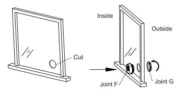
3. Install the other side of heat discharge pipe clockwise into joint F.
