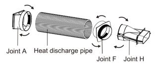
3.Insert joint A of heat discharge pipe (the side with "TOP" is upwards) into the groove until you hear a sound.
