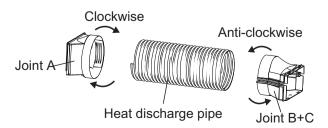
9. Insert joint A of heat discharge pipe (the side with "TOP" is upwards) into the groove until you hear a sound.
