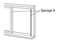
3. Install the window panel into the window frame.
