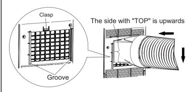
3. Insert the joint E into the wall, fix it with screws and then rotate the joint D into joint E.
