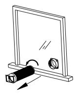
3. When heat discharge pipe is removed, Install the plastic cover into joint F in case of the insect into the house .
