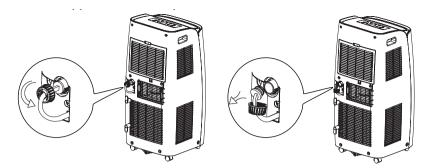
(2) Screw the drain connector to(included in the package) the spout by turning clockwise.
