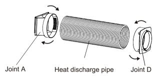
2. Insert joint A of heat discharge pipe (the side with "TOP" is upwards) into the groove until you hear a sound.
