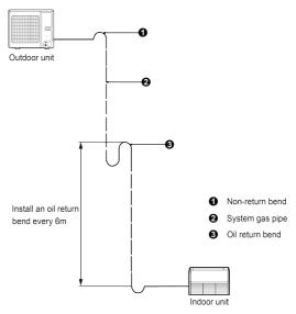
Dimensions for the making of oil return bend are as follows:
