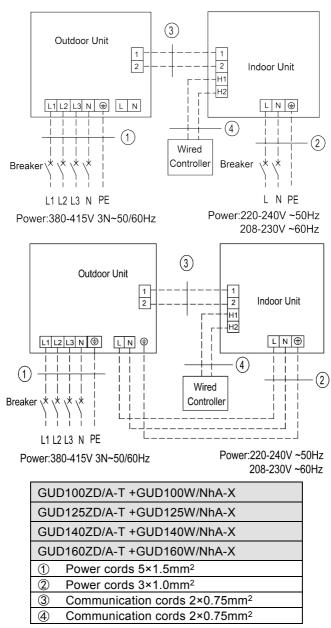
(5) Electrical wiring of indoor unit and Electrical wiring of outdoor unit.
