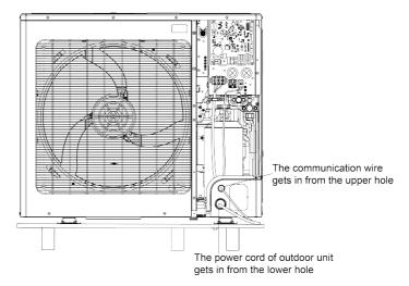
B. Wire routing of unified power supply for single phase.
